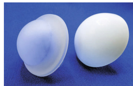
Complex curved MgAl_2O_4 ceramic with different wall thicknesses (left) and curved Al_2O_3 ceramic (right).
