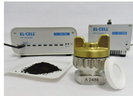
Measuring cell with sodium-beta alumina and transition metal oxide active material (Source: EL-CELL).
