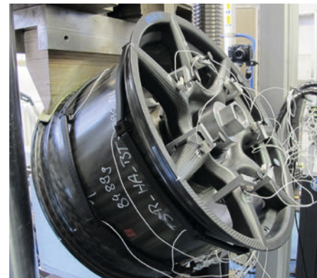
CfK rim testing with acoustic emission analysis.
