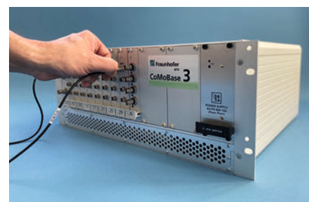
Acoustic measurement system with 32 channels.
