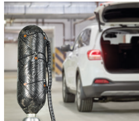
Permanent monitoring of pressure tanks with guided waves.
