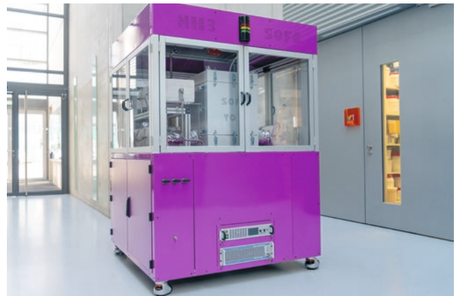
Figure 2: NH 3 -SOFC demonstration plant.
