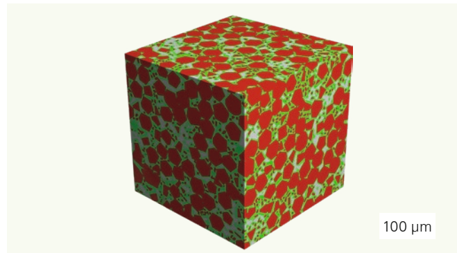
Figure 2: Artificially generated 3D microstructure of a diamond-SiC composite as a basis for simulating thermal properties.
