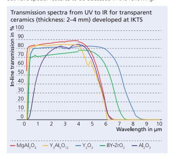
Due to their polycrystalline structure, the transmission in ceramics is influenced by stray light of pores and foreign phases. In anisotropic crystal systems (such as corundum and tetragonal  $\rm ZrO_2$ ), additional scattering of light by the directional dependence of the refractive index, which leads to a splitting of
