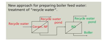
The 19-channel NF membranes showed rejection of alkaline earth metals (Ca and Mg) of up to 80 % and of alkali metals (Na and K) of up to 55 %. The permeate was free of organic matter. Long-term tests performed over several months confirmed the stability of the membranes.
