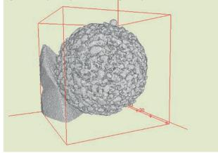
shows the three-dimensional visualizations of an Al<sub>2</sub>O<sub>3</sub> granule recorded by X-ray nanotomography. A FIB tomography generated structure belonging to the same granule batch is shown in Figure 2A and 2B.
