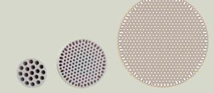
In lab measurements, the membranes showed the same flux and retention behavior as that of 19-channel NF membranes.
