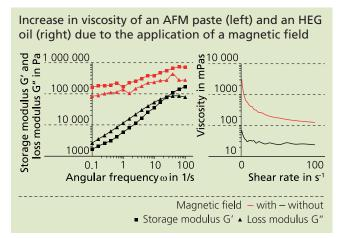
Due to the switchable strong increase in solidity (see diagram), a significant and specific increase of material removal efficiency is expected in both machining processes.
