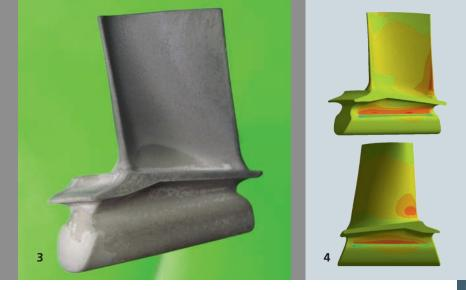
greatest challenge proving to be the debinding process. This problem was solved by an innovative combination of chemical and thermal treatment of the part to enable sintering of defect-free rotors.
