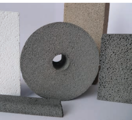
Direct-foamed ceramic components made of various materials with different porosities.
