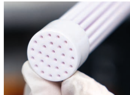
Ceramic capillary membranes with hydrophobic surface coating.
