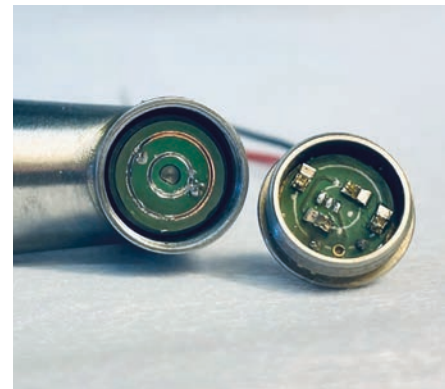
Miniature slip ring based on a circuit board.
