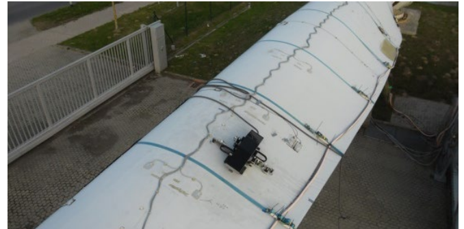
Ultrasonic scanning carriage during a diagnostic scan on a rotor blade.
