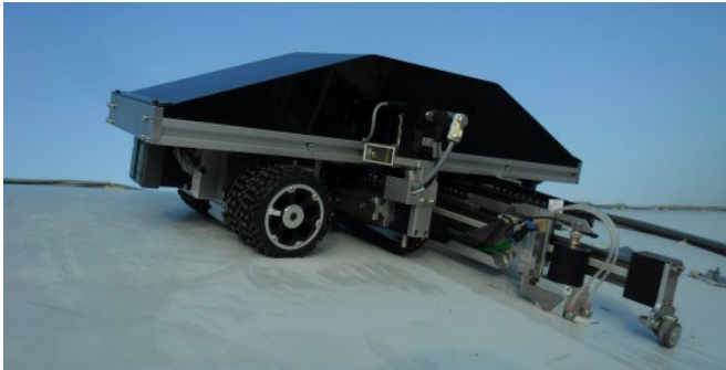
Scanning carriage on a rotor blade surface
