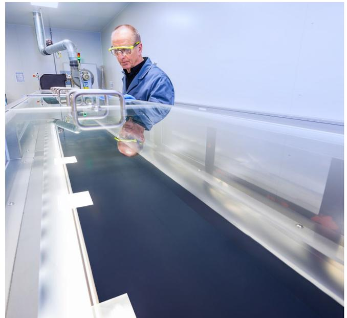
*Electrode production for Li-ion battery.*
