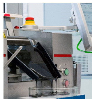
Final homogenization of a paste on a three-roll mill.
