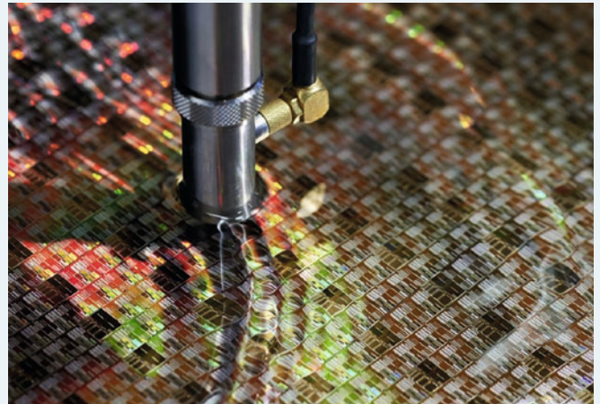
A wafer being scanned by an ultrasonic probe.
