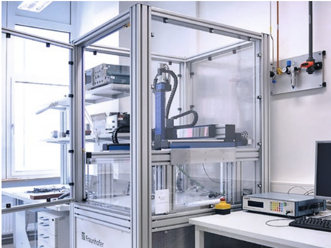
Lab system of the VARIUS ultrasonic scanner for detecting hollow spaces and cracks in weld seams and glued joints and other faults in composite materials.
