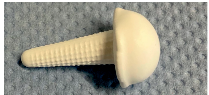
Slip-cast patient-specific implant made of ATZ.
