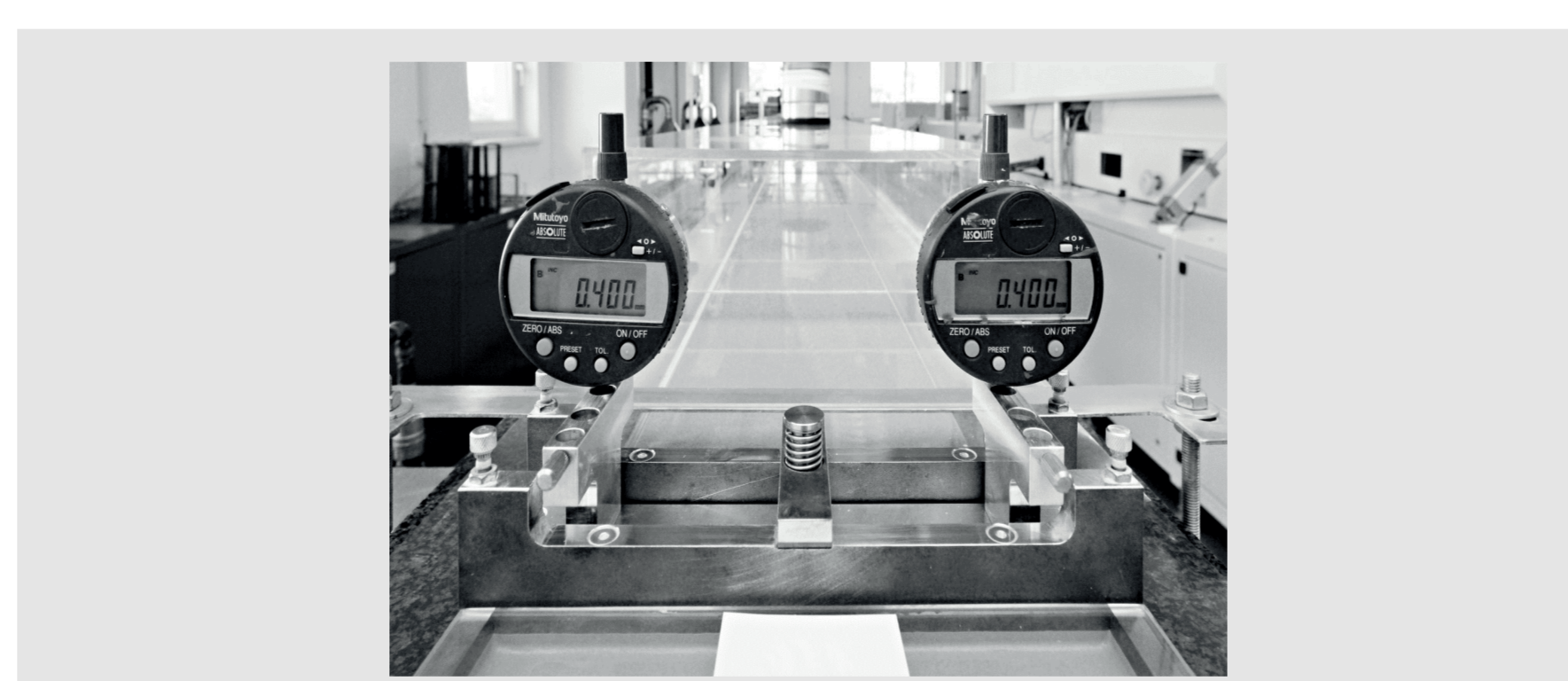
Figure 7: Tape caster “KWH”, View from the front end into the drying channel
