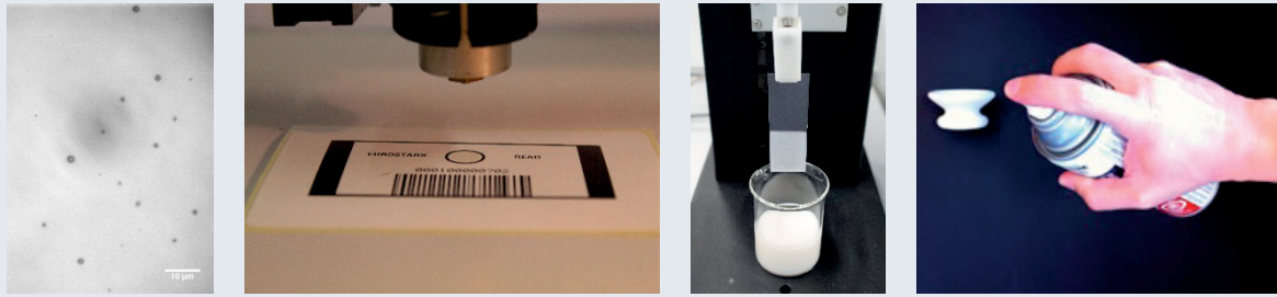
Figure 2 Examples of deposition techniques for the dosimetric active ceramic phosphor. From left to right: embedding, nozzle printing, dip coating, spraying.
